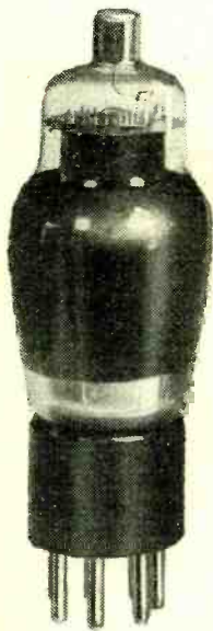
6A7 Pentagrid with a heater rated at 6.3 volts 0.3 ampere.
